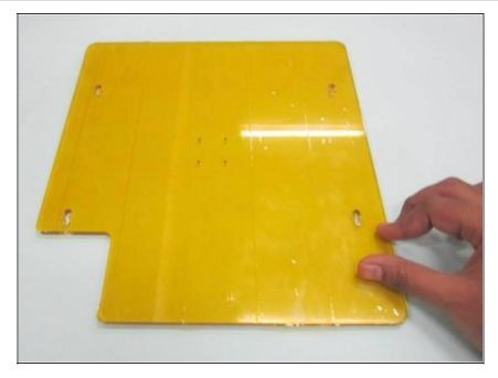
Use fingers and press tape against print plate. We do it to avoid air bubbles in between kapton tape and print plate.
