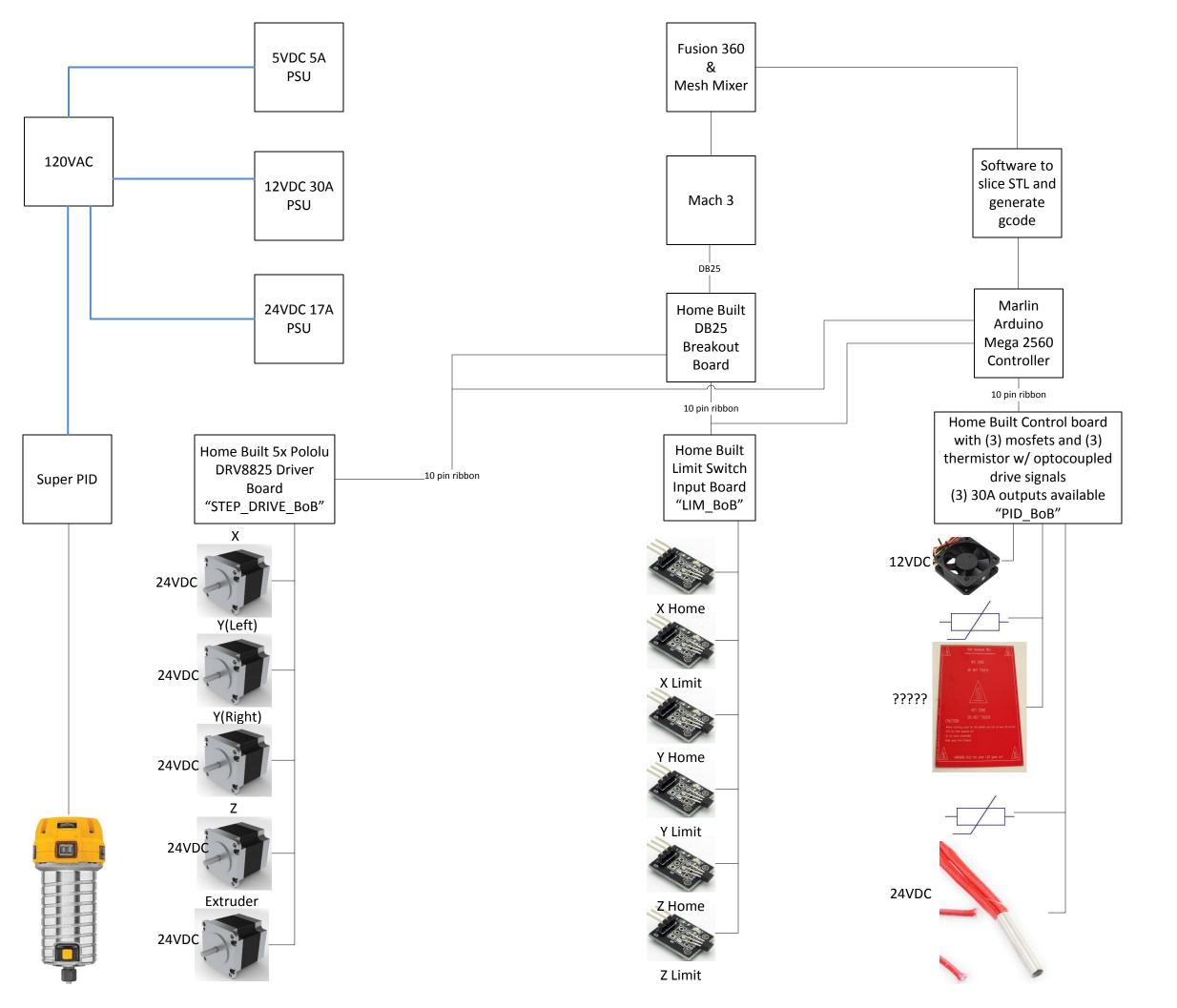
Shapeoko 2 CNC/3D Printer System Arch.
