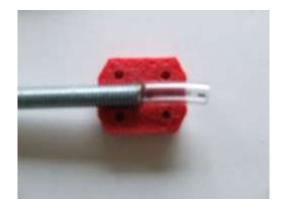
Fix extruder to X carriage with M4x20mm bolts 2 bolts, 2 washers and 2 nuts.
