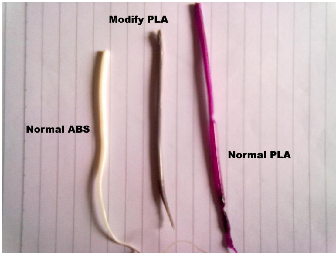
Pic 1 PLA filament were pull out from extruder
