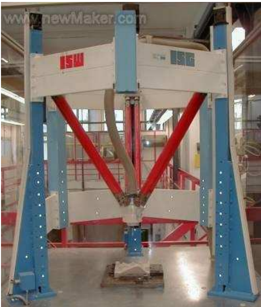
A different configuration but still a triaglide, the working area can be tailored to suite the application. You can again see a pair of struts on each axis to keep the tool pointing down.
