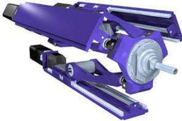
Fig. 2: The Sprint Z3 PKM tool head by DS Technologie GmbH.
