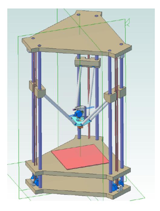
Printing Volume: 200x200x H=230. Printing design speed: 80mm/sec. Printing design positioning accuracy: 0.05 mm Hot plate foreseen Build in progress 01-09-2014
