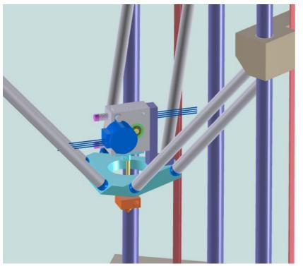
Lo=49 mm and a steel wire d=0.3 mm centered in between a pair of Arms. (~25 N pulling force)
