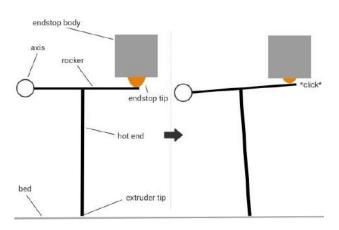
Figure 1: Mechanical scheme of the mechanism after and before switching.
