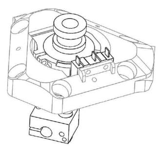
Figure 6: 3D view of my design of delta head.
