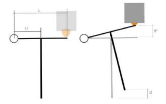
Figure 2: Geometric parameters of the mechanism, d and  $d^*$  represent distances at the moment of end-stop switching.
