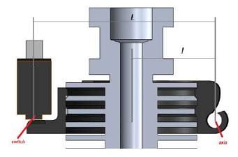
Figure 3: Section view of my implementation of this mechanism of my own 3D printer.
