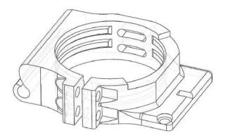
Figure 7: 3D view of the Rocker/Clamp.
