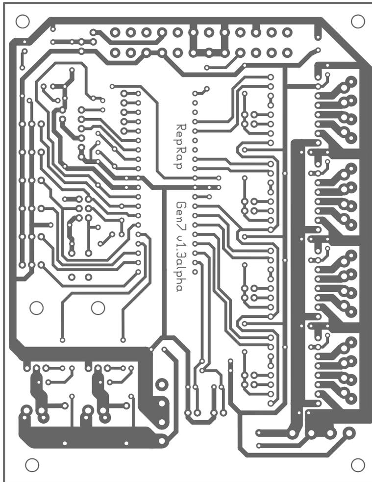
There are 5 different drill sizes used in this layout, 357 holes total
