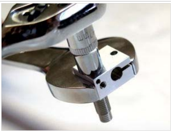
A first, slight tightening of the nozzle against the break.
