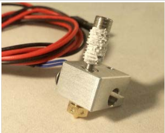
Thermal compound spread over the threads of the heat-break.
