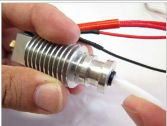
PTFE Tubing being pushed down into HotEnd.
