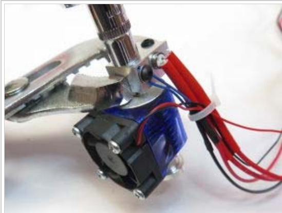
Doing the final tightening of the nozzle.
