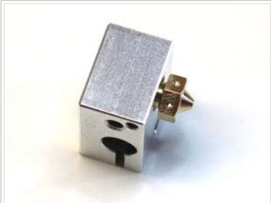
Nozzle screwed into block, and unscrewed a 1/2 turn.
