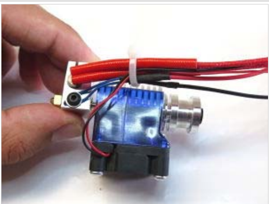
Cable tie all wires together.
