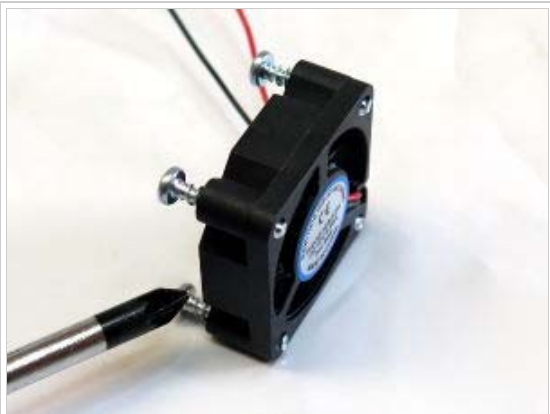
Fan with screws inserted.
