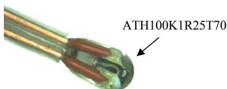
Figure 4.2. Tubing Ledged Non-sealed Thermistor Head Photo
