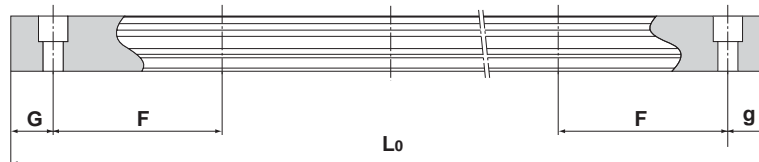
Standard Length and Maximum Length of the LM Rail for Model HSR with Ct Grade
