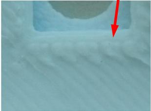
nozzle is pushing the material to early so when he is printing a line there is to much material at the start point
