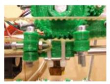
Rod clamps use M3x 20mm 4 bolts, 4 washers and 4 nuts
