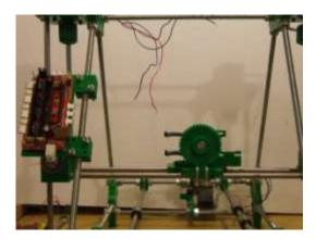
Fix Z couplings to motor shafts and threaded rod with M3x20mm bolts 8 bolts, washers and nuts. Put 5mm tube on the Z motor shafts.
