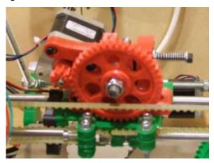
Fix gears to motor shafts, (file a flat on the shaft) with M3 grub screws and capture nuts inserted into the gear.
