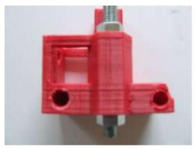
Use M3x16mm bolts for the 40mm fan bolted to the X carriage (insert the nuts before the bearings as they need a tap down with a hammer).
