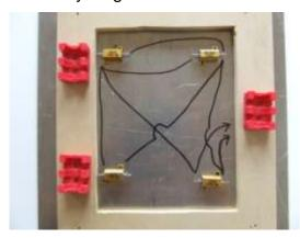
Fix housed resistors to aluminium with countersunk M3x10mm bolts 8 bolts and nuts
