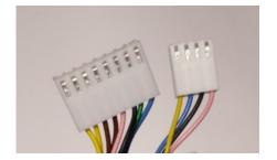
10. Optionally, add a 4th wire back to the Ormerod. You only need this wire if you want to be able to use the backup mode (simple modulated IR sensor), for example if you have difficulty with x-homing when using the differential IR sensor.
