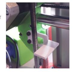
9. The 4-way connector is for the sensor loom. Cut off the existing 3-way sensor connector from the sensor loom, strip the ends of the wires, attach the crimp receptacles supplied, and push them into the correct positions in the 4-way shell (see photo). Ignore the yellow wire on the 4-pin connector in the photo. Your wiring loom may have a red wire instead of the pink wire shown, and it may have two orange wires instead of two brown wires.
