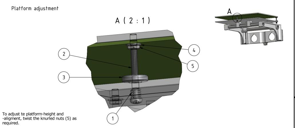
The M3 nut (4) fastens the M3 bolt (2) to the top-platform. The knurled nut (5) adjusts the distance between bottomand top-platform.
