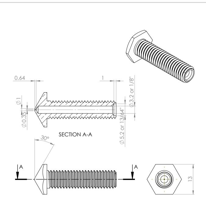
Can be manufactured form Hex Bar or from a Brass M8x30mm Hex bolt
