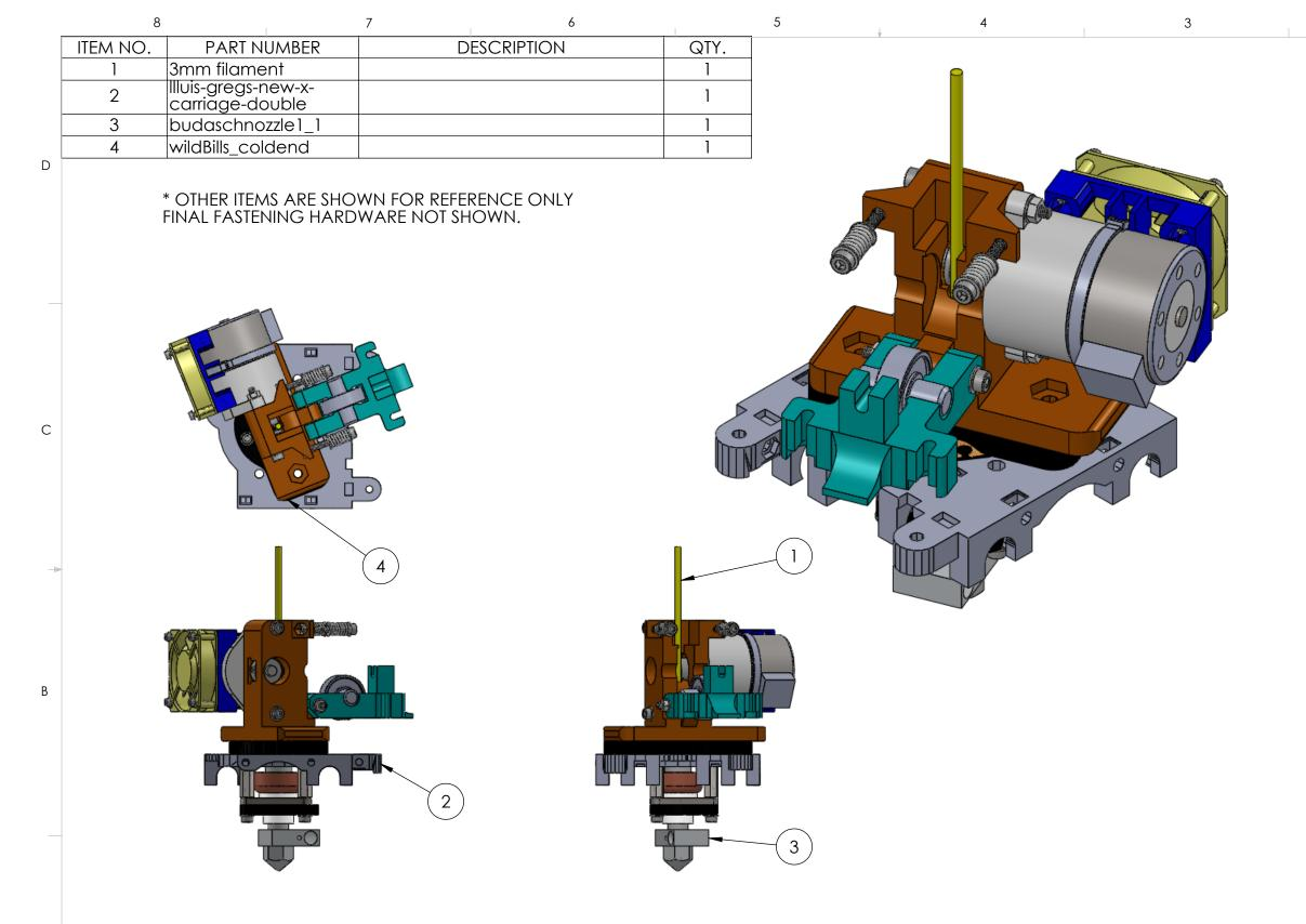
RECOMMENDED MOUNTING ORIENTATION TO AVOID HITTING THREADED RODS.
